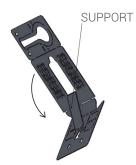
STEP 4- ROTATE THE SUPPORT UNTIL THE HOOK IS INSERT INSIDE THE GAP
