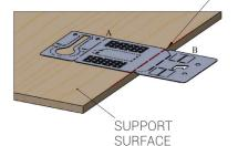
STEP 1- LAY THE SURFACE "A" OF THE PLATE ON A FLAT SURFACE, LEAVING SURFACE "B" PROTRUDING
