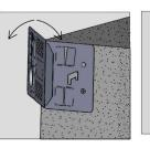
STEP 6 – REMOVING THE EXCEEDING OF PART OF THE PLATE SWINGING IT UNTIL IT IS COMPLETELY REMOVED
