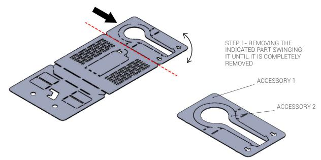
STEP 2- PRESS ON THE INDICATED PART UNTIL THE TWO ACCESSORIES ARE SEPARATED
