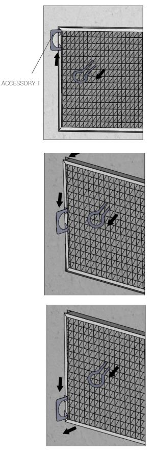
STEP 4- SLIDE ACCESSORY 1 UPWARD UNTIL THE TOP OF THE GRILLE IS RELEASED
