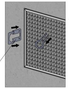
STEP 3- INSERT ACCESSORY 1 LATERALLY BETWEEN GRILLE AND WALL, UNTIL THE FOLDED PART IS FLAT
