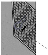
STEP 1- PUT ACCESSORY 2 INSIDE THE CRATE GRILLE UNTIL THE HOOK ARE LOCKED
