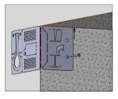
STEP 5- DRILL THE MASONRY AND FASTEN THE PLATE WITH SCREW/S AND DOWEL/S TO BE PLACED AS IN THE PICTURE
