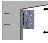
STEP 7- FASTEN THE SCREWS INTO THE DRYWALL PLATE UNTIL THE SLOTTED HOLES IN THE PLATE ARE REACHED
