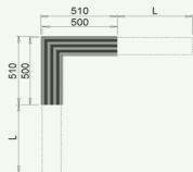
Data referring to 1m long diffusers, with a terminal throw velocity Vt=0.25 m/s and with a temperature differential of 10/12°C, in ceiling installations and with lateral air throw.
